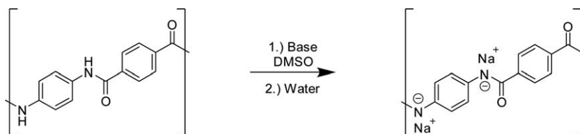
Scheme 1. Overall reaction of the hydride-based method for achieving ANF dispersions. The addition of water to the highly basic DMSO solution was believed to complete the dispersal process due to hydroxyl anion formation.
